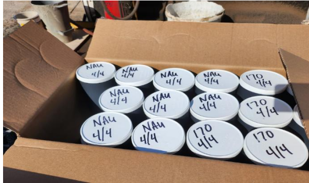
Figure 16: Fabricated test cylinders in molds
